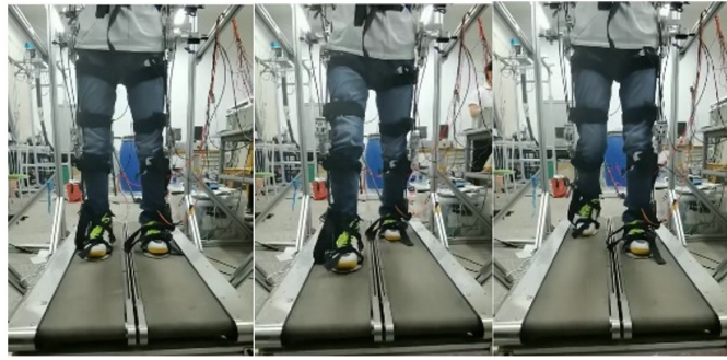
Fig. 6. Lower limb exoskeleton walking test
